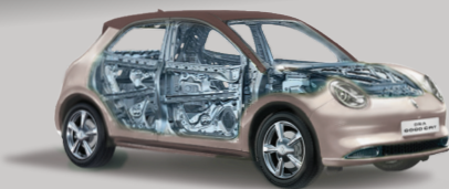
65% High Strength Steel Throughout Vehicle Body
