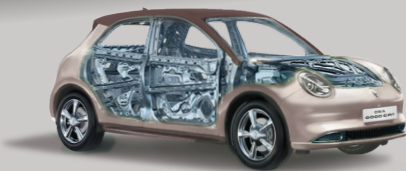
65% High Strength Steel Throughout Vehicle Body
